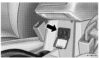
Power Outlet — 115 Volts (150 Watts)
